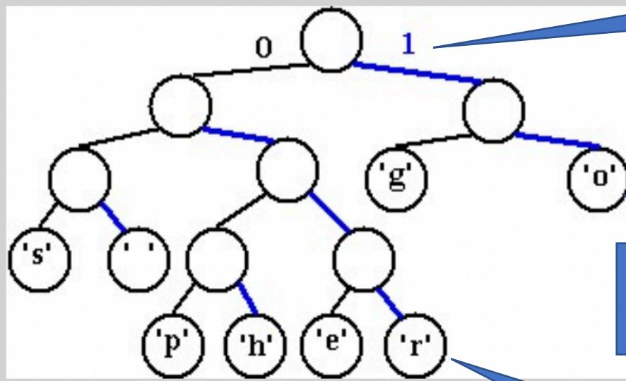
Encoding is the sequence of 0's and 1's on root to leaf path
