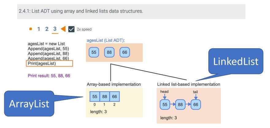
A list ADT is commonly implemented using array and linked list data structures. But, a programmer need not have knowledge of which data structure is used to use the list ADT.
