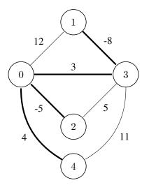
Above, the 5-vertex graph G represented by the matrix M below. The thick edges denote the (unique) MST in G, which has total cost -6.
