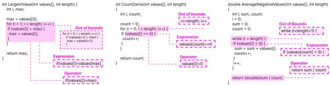
Figure 1: The three examples of code with the correct variant, and the three incorrect variants annotated. The incorrect variants were 1) operator error, 2) expression error, and 3) out-of-bounds error.
