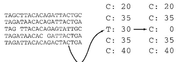
**Figure 1** Correcting errors in reads. A portion of a multiple alignment between five reads is shown. In the highlighted column of the alignment, a base T of quality 30 is aligned only to bases C, some of which are of quality greater than 30. The base T is changed to a base C of quality 0.
