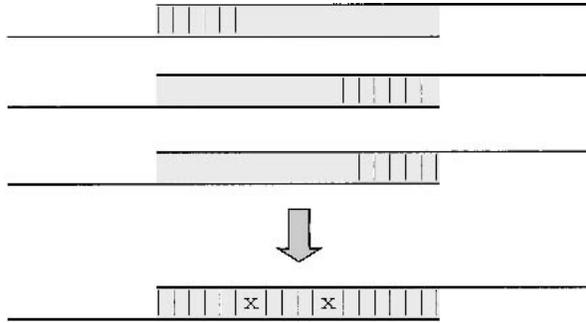
**Figure 8** Partial alignments in the alignment module. Three partial alignments of length  $k = 6$  between a pair of reads coalesce to yield a single full alignment of length  $k = 19$ . Vertical bars denote matching bases, whereas  $x$ 's denote mismatches. This illustrates the commonly occurring situation where an extended  $k$ -mer hit is a full alignment between two reads ( $k = 6$  is used in the figure for simplicity).
