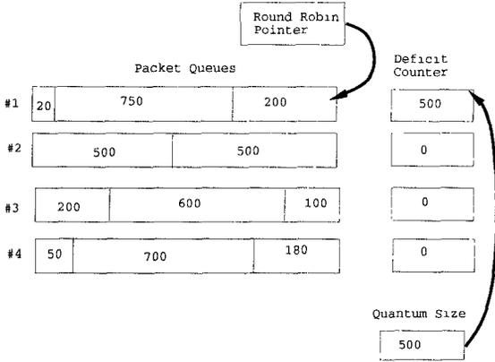
Figure 2: Deficit Round Robin: At the start, all the *DeficitCounter* variables are initialized to zero. The round robin pointer points to the top of the active list. When the first queue is serviced the *Quantum* value of 500 is added to the *DeficitCounter* value. The remainder after servicing the queue is left in the *DeficitCounter* variable.
