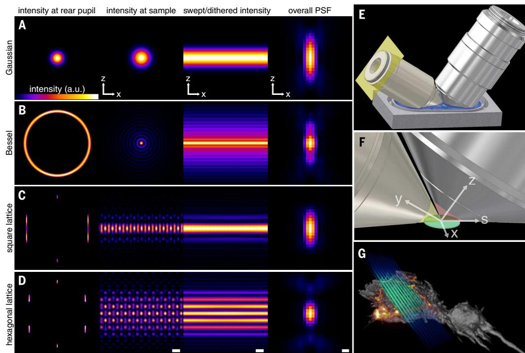
lattice light sheet as a binary phase pattern on the SLM (fig. S5). Incident laser light is then diffracted by the SLM, filtered by the mask, and focused by the excitation objective to produce a light sheet and corresponding PSFs in good agreement with theoretical predictions (fig. S6).
