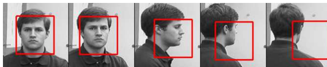
Figure 2: A series of images demonstrating the drift that can take place during tracking.
