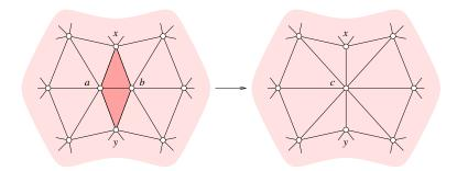
Figure II.9: To contract ab we remove the two dark triangles and repair the hole by gluing their two left edges to their two right edges.
