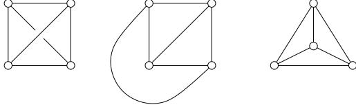
Figure 73: Three drawings of  $K_4$ , the complete graph with four vertices. From left to right: a drawing that is not an embedding, an embedding with one curved edge, a straight-line embedding.
