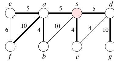
Figure 59: The bold edges form shortest paths and together the shortest path tree with root  $s$ . It differs by one edge from the breadth-first tree shown in Figure 57.
