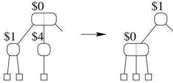
Figure 32: The underflowing node is merged with a sibling and the parent is treated recursively.
