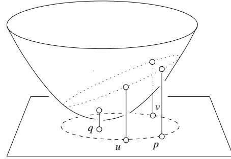
Figure 103: The plane passing through  $u^+, v^+, p^+$  intersects the paraboloid in an ellipse whose projection into  $\mathbb{R}^2$  passes through the points  $u, v, p$ . The point  $q^+$  lies below the plane iff  $q$  lies inside the circle.
