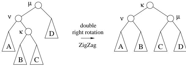
Figure 19: The double right rotation at  $\mu$  is the concatenation of a single left rotation at  $\nu$  and a single right rotation at  $\mu$ .
