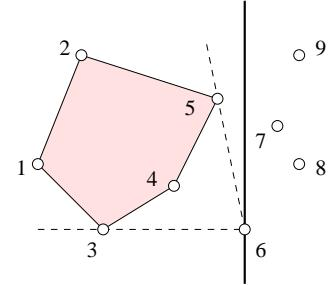
Figure 92: The vertical sweep-line passes through point 6. To add 6, we substitute 6 for the sequence of vertices on the boundary between 3 and 5.
