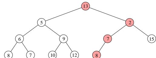
Figure 41: The root is exchanged with the smaller of its two children. The operation is repeated along a single path until the heap-order is repaired.
