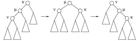
Figure 35: If in the middle tree the balance of  $\nu$  is the same as the balance of  $\mu$  then by the Balance Lemma the balance of  $\kappa$  is less than that common balance.
