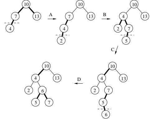
Figure 20: Sequence of red-black trees generated by inserting the items 10, 7, 13, 4, 2, 5, 6 in this sequence.
