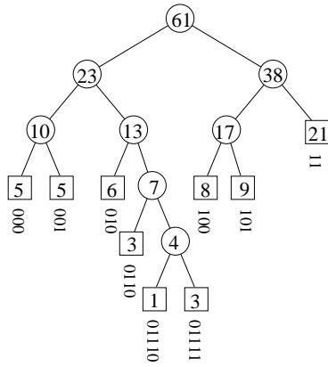
Figure 9: The weighted external path length is  $15 + 15 + 18 + 12 + 5 + 15 + 24 + 27 + 42 = 173$ .
