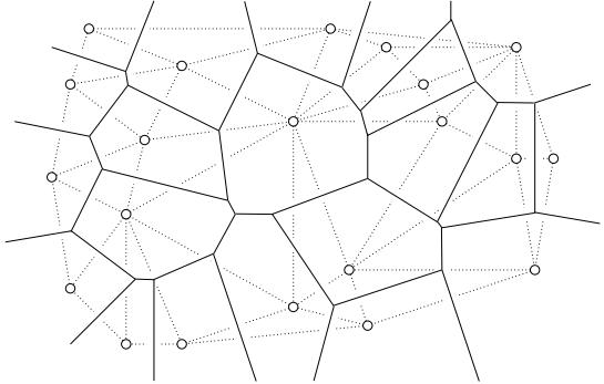
Figure 99: The (solid) Voronoi diagram drawn above the (dotted) Delaunay triangulation of the same twenty-one points triangulated in Figures 97 and 98. Some of the Voronoi edges are too far out to fit into the picture.
