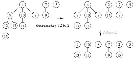
Figure 48: A Fibonacci heap initially consisting of three binomial trees modified by a decreasekey and a delete operation.
