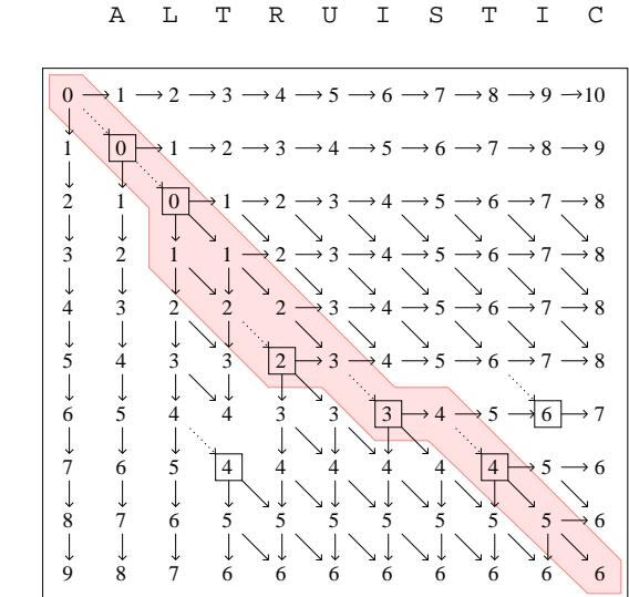
Figure 5: The table of edit distances between all prefixes of ALGORITHM and of ALTRUISTIC. The shaded area highlights the optimal edit sequences, which are paths from the upper left to the lower right corner.
