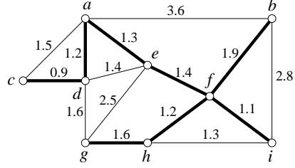
Figure 64: The bold edges form a spanning tree of weight  $0.9 + 1.2 + 1.4 + 1.1 + 1.2 + 1.6 + 1.9 = 10.6$ .
