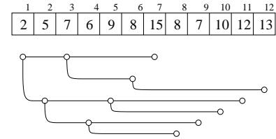
Figure 40: The binary tree is layed out in a linear array. The root is placed in  $A[1]$ , its children follow in  $A[2]$  and  $A[3]$ , etc.
