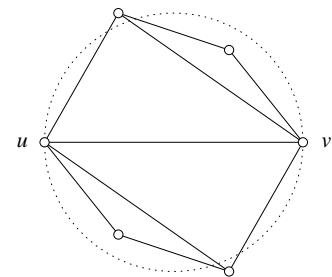
Figure 101: The edge  $uv$  is locally Delaunay but does not belong to the Delaunay triangulation.
