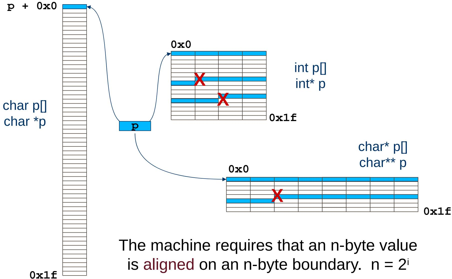
The machine requires that an  $n$ -byte value is aligned on an  $n$ -byte boundary.  $n = 2^i$
