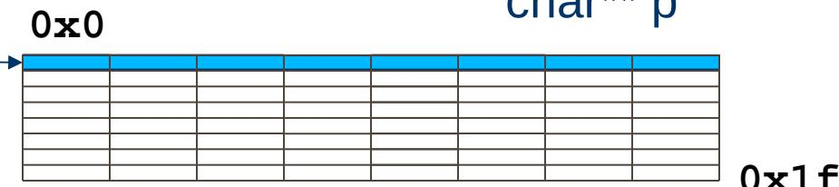
Pointers (addresses) are 8 bytes on a 64-bit machine.
