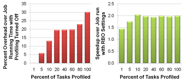
Figure 10: (a) Overhead to measure the (approximate) profile, and (b) corresponding speedup given by CBO over RBO as the percentage of profiled tasks is varied for Word Co-occurrence.
