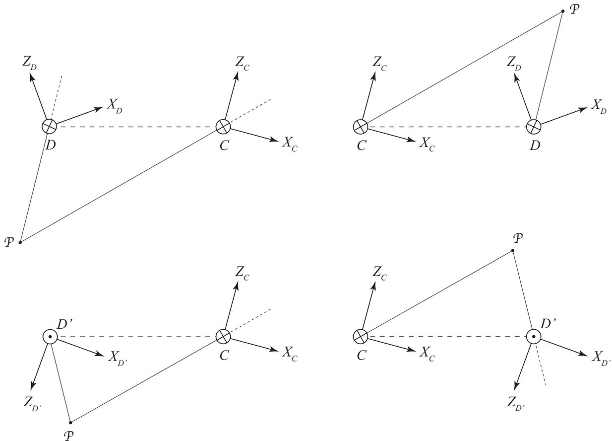
Figure 3: The fourfold ambiguity of reconstruction corresponds to the two ways to pick the sign of  $\mathbf{t}$  (left or right diagrams) and the two ways to choose the rotation matrix  $R$  (top or bottom diagrams). A circle with a cross (a dot) denotes a  $Y$  axis pointing into (out of) the page. Only the arrangement in the top right has the scene structure (represented by the single point  $\mathbf{P}$  and its two projection rays) in front of both cameras.
