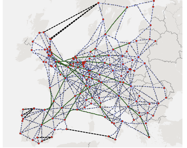
Fig. 13: A 100 Gbps 1.04\times stretch cISP across Europe. This network uses several fiber connections (dashed, black lines).
