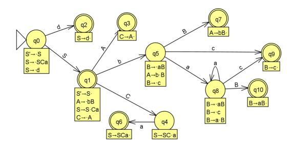
(a) In processing some string, suppose you have reached the state  $q_3$ . After processing the reduce operation  $C \to A$  which possible state(s) could you be in? Give the path(s) that reached that state(s). If path but for  $q_1$ , for  $q_2$
