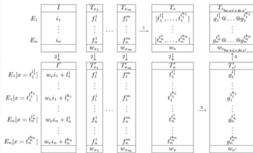
Figure 6: TRANSLATION OF "for x \in e do e' " IN THE ENVIRONMENT FOR x_1, \dots, x_m .
