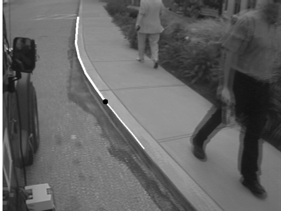
Figure 7 Image taken by the right forward-looking camera. Overlaid is the current curb position detected by the line striper (black dot), the curb position tracked 1 m alongside the vehicle, and the curb detected in front of the vehicle using this image.
