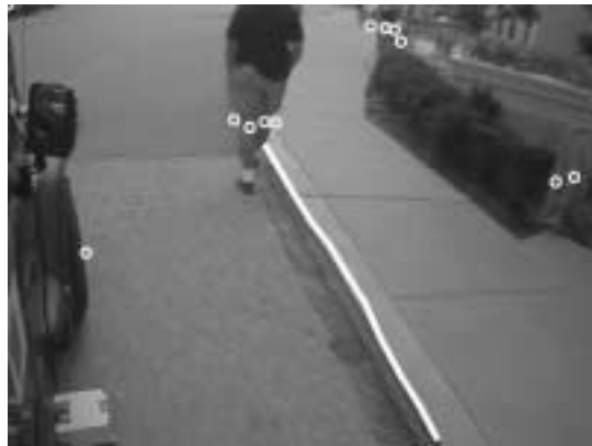
Figure 8 Obstacle in front of the curb. The laser scanner detects the obstacle (white circles) and the search of the curb in front of the vehicle stops when it reaches the object.
