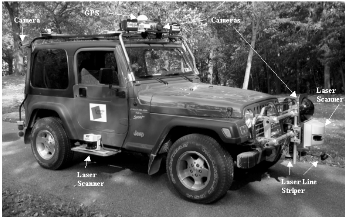
Figure 1: Navlab 11 testbed showing cameras, GPS, Laser Scanners, and a Laser Line Striper (one arrow points to the laser, the other to the camera). On the left side of the vehicle is another camera and Laser Scanner, positioned symmetrically to the ones on the right side.
