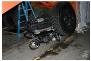
Figure 7. Typical steering offset causing crash
