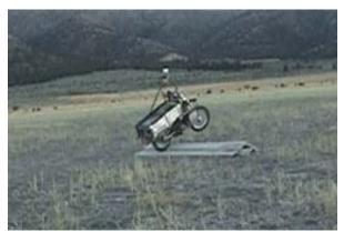
Figure 5. Testing of ability to run on bumpy terrain
