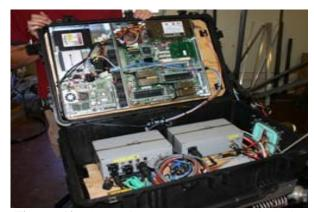
**Figure 10.** Supermicro SuperServer Dual Code AMD Opteron
