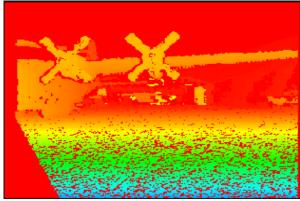
**Figure 17.** Image of 3D reconstruction with low rejection note invalid background measurements. Color represents distance
