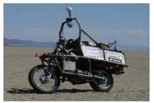
**Figure 12.** Topcon Map HP receiver on top of Ghostrider during endurance test in Nevada
