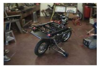
Figure 18. Testing of self-righting arms
