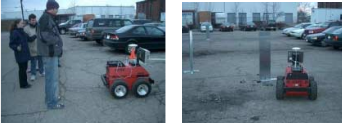
Figure 4. The test robot with GPS and Lidar in the GC Design Course at OSU.
