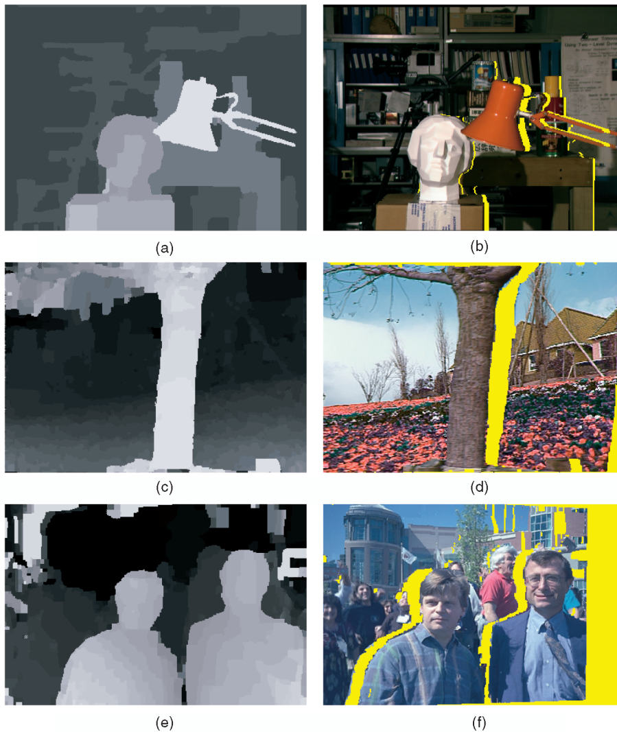
Fig. 11. The results of multiview stereo. (a), (c), and (e) are depth maps. (b), (d), and (f) are novel views rendered. (a) Our result (3rd frame). (b) Novel view. (c) Our result (6th frame). (d) Novel view. (e) Our result (3rd frame). (f) Novel view. (Yellow regions are disocclusion regions. Please refer to the electronic version for better quality viewing.)
