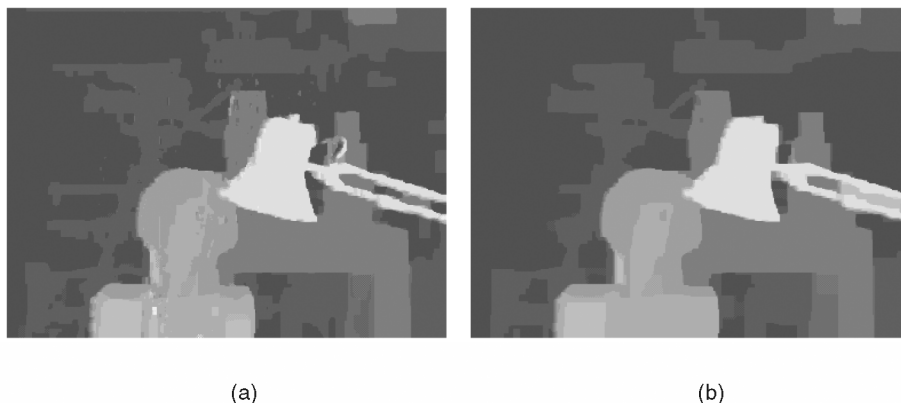
Fig. 12. (a) Result of TV model ( B_O = 2.16 , B_T = 1.01 , B_{DD} = 11.67 ). (b) Result of Gaussian model ( B_O = 2.82 , B_T = 1.58 , B_{DD} = 15.14 ). The results obtained by TV model \rho_p(d_s, d_t) = \frac{|d_s - d_t|}{\sigma_p} and Gaussian model \rho_p(d_s, d_t) = \frac{|d_s - d_t|^2}{\sigma_p} . The parameter \sigma_p is chosen experimentally to produce the best result for each model.
