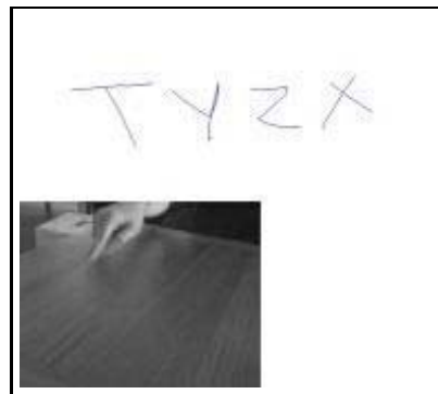
Figure 7: Using 3D tracking of the finger tip as a virtual mouse to control a drawing application. Inset shows left image view.
