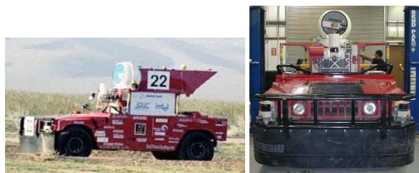
Figure 6: CMU's Sandstorm autonomous vehicle. TyzX DeepSea Stereo sensor is mounted in the white dome.
