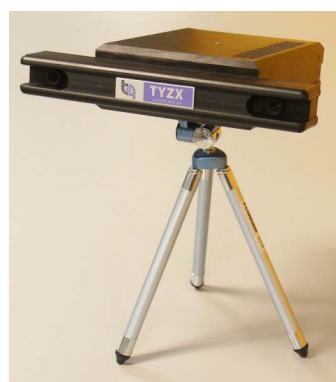
Figure 8: TyzX Integrated Stereo System. Self contained stereo camera, processor, and general purpose CPU.
