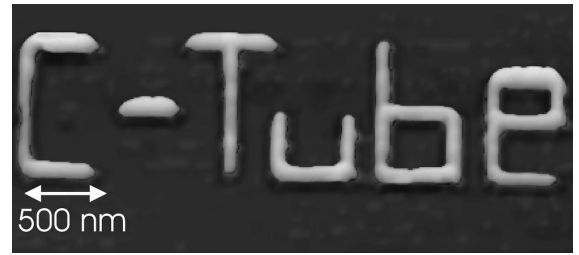
Fig. 11. Use of conducting carbon nanotube AFM tips as nanofabrication tools. In this case, a nanotube-bundle tip was used as the negative electrode to locally oxidize silicon and write the oxide pattern ‘C-Tube’.
