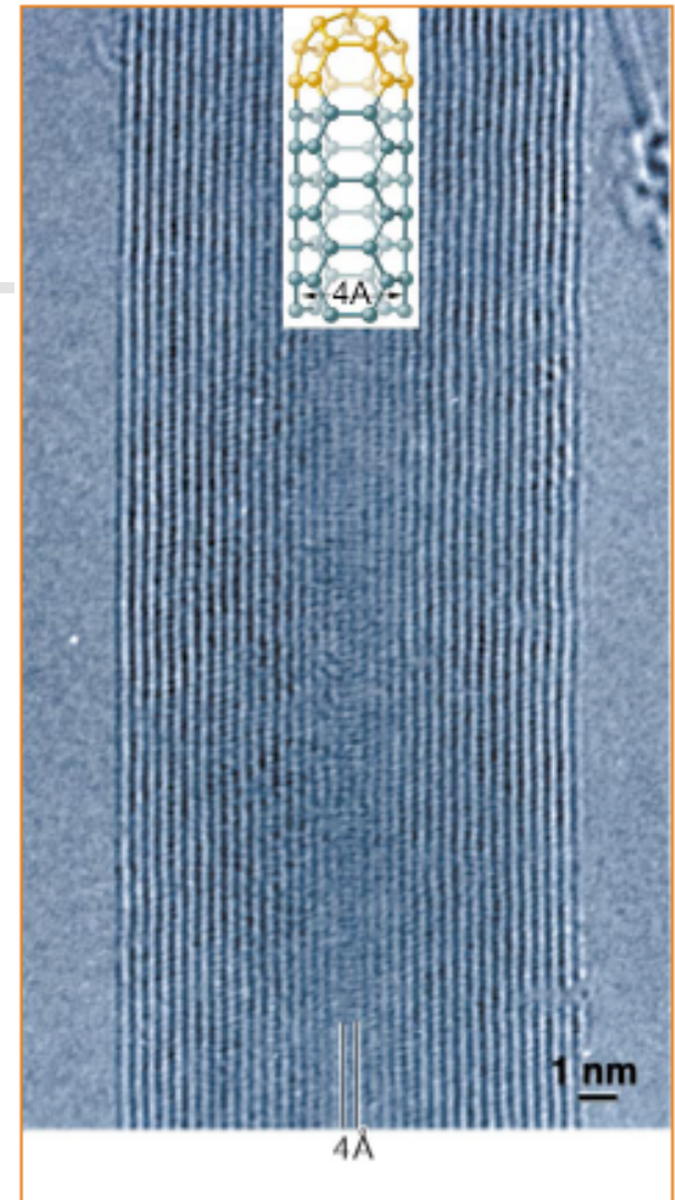
Figure 1 High-resolution electron microscope image of a 4 Å tubule (side walls are marked by lines) confined inside an 18-shell carbon nanotube. Dark lines correspond to the side
