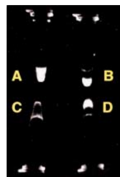
Figure 4. Black-and-white photograph of samples under UV irradiation: A) mutant CPMV- 3 conjugate + stilbene-binding antibody 19G2; B) denatured mutant CPMV- 3 conjugate + 19G2; C) wild-type CPMV- 3 conjugate + 19G2; D) denatured wild-type CPMV- 3 conjugate + 19G2. Note that denaturation causes precipitation of the viral protein, but exposed stilbenes are still recognized by the antibody.
