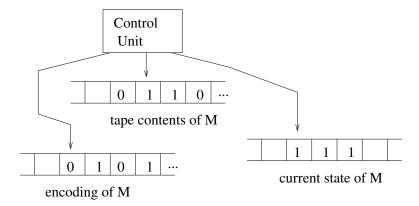
Tape 1 contains the encoding of a TM M. Tape 2 contains the contents of the tape of M. Tape 3 contains the current state.
