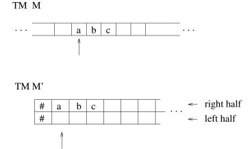
• ( $\Leftarrow$ ): Given a TM M with semi-infinite tape there exists a standard TM M' such that L(M)=L(M').
