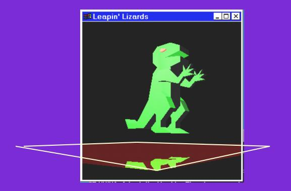
Clear stencil to zero. Draw floor polygon with stencil set to one. Only draw reflection where stencil is one.
