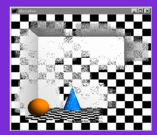
Stencil buffer holds dissolve pattern. Stencil test two scenes against the pattern
