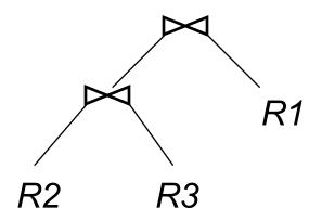
Optimal for joining *R1*, *R2*, *R3*
