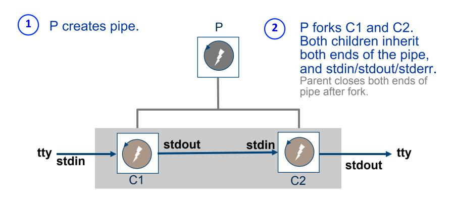
C1 closes the read end of the pipe, closes its stdout, "dups" the write end onto stdout, and execs.
