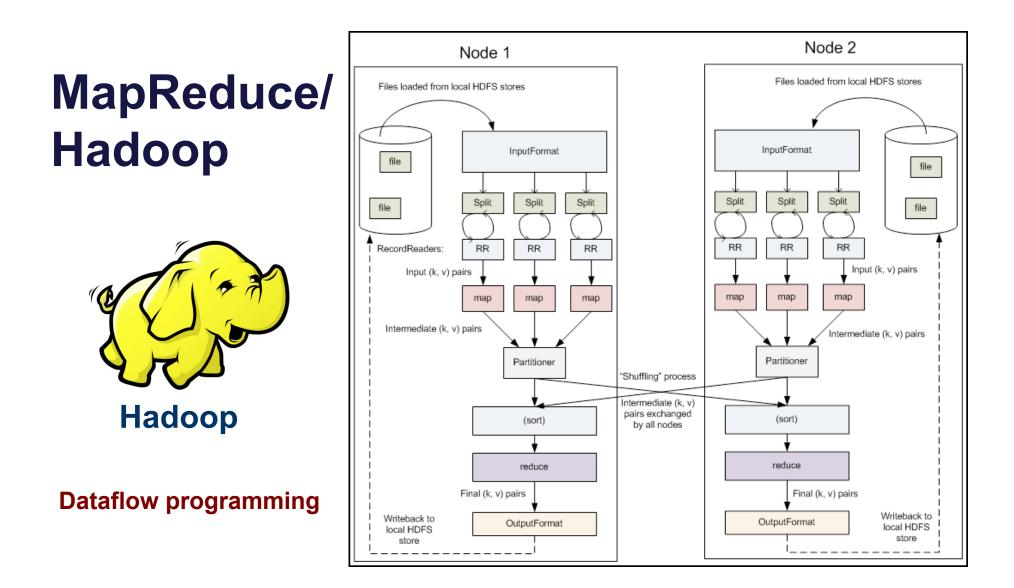
**MapReduce** is a filter-and-pipe model for **data-intensive cluster computing**. Its programming model is "like" Unix pipes. It adds "parallel pipes" (my term) that split streams among multiple downstream children.
