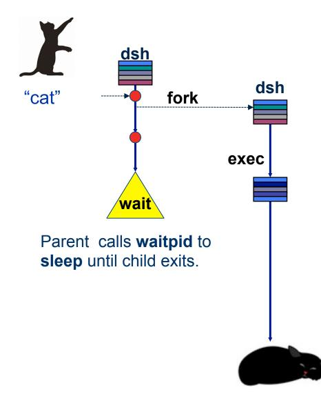
**dsh** runs in child to initialize kernel state and launch the program. The child inherits stdin and stdout bound to the controlling terminal.
