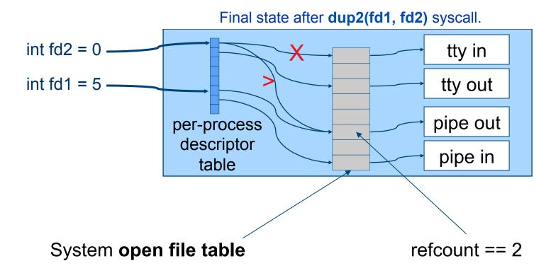
Why should you close(fd1) after dup2(fd1, fd2)? Because the kernel uses reference counting to track open file descriptors. Resources associated with an I/O object are not released until all of the open descriptors on the object are closed. They are closed automatically on exit, but you should always close any descriptors that you don't need.
