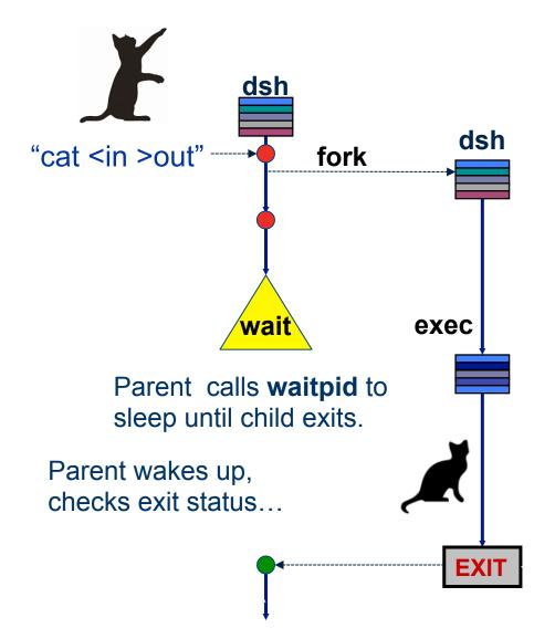
Child process running **dsh**: it is a clone of the parent, including a snapshot of parent's internal data (from parser, etc.), and any open descriptors, current directory, etc.
