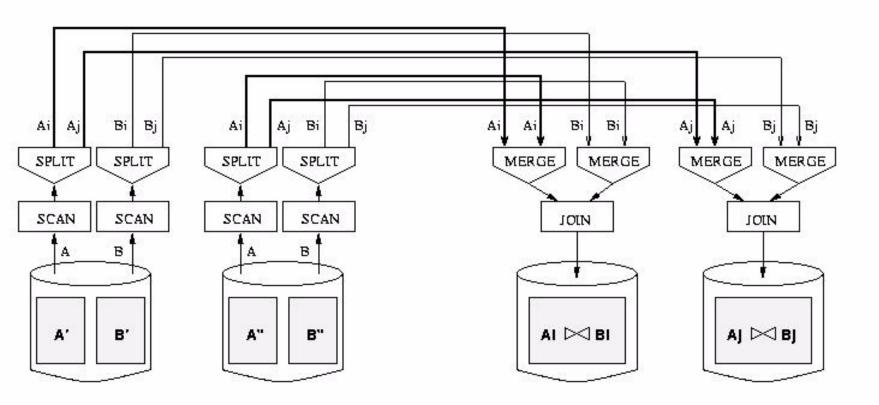
Good use of split/merge makes it easier to build parallel versions of sequential join code.
