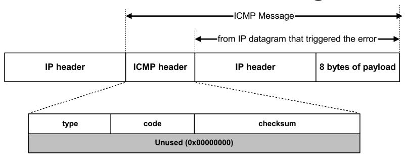
• ICMP error messages include the complete IP header and the first 8 bytes of the payload (typically: UDP, TCP)
