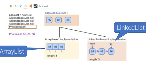
A list ADT is commonly implemented using array and linked list data structures. But, a programmer need not have knowledge of which data structure is used to use the list ADT.
