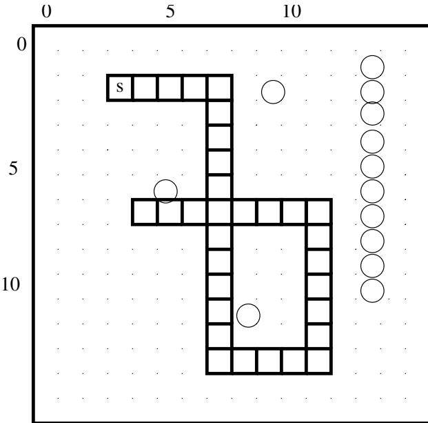
In the picture, single obstacles (denoted as circles) are drawn in positions (8,11), (9,2), (5,6), and a wall of obstacles from (13,1) to (13,10). The robot rob starts in position (3,2) (denoted by the s in the square) and the robots movements are indicated by the squares. In this example, the robot safely avoided all the obstacles.
